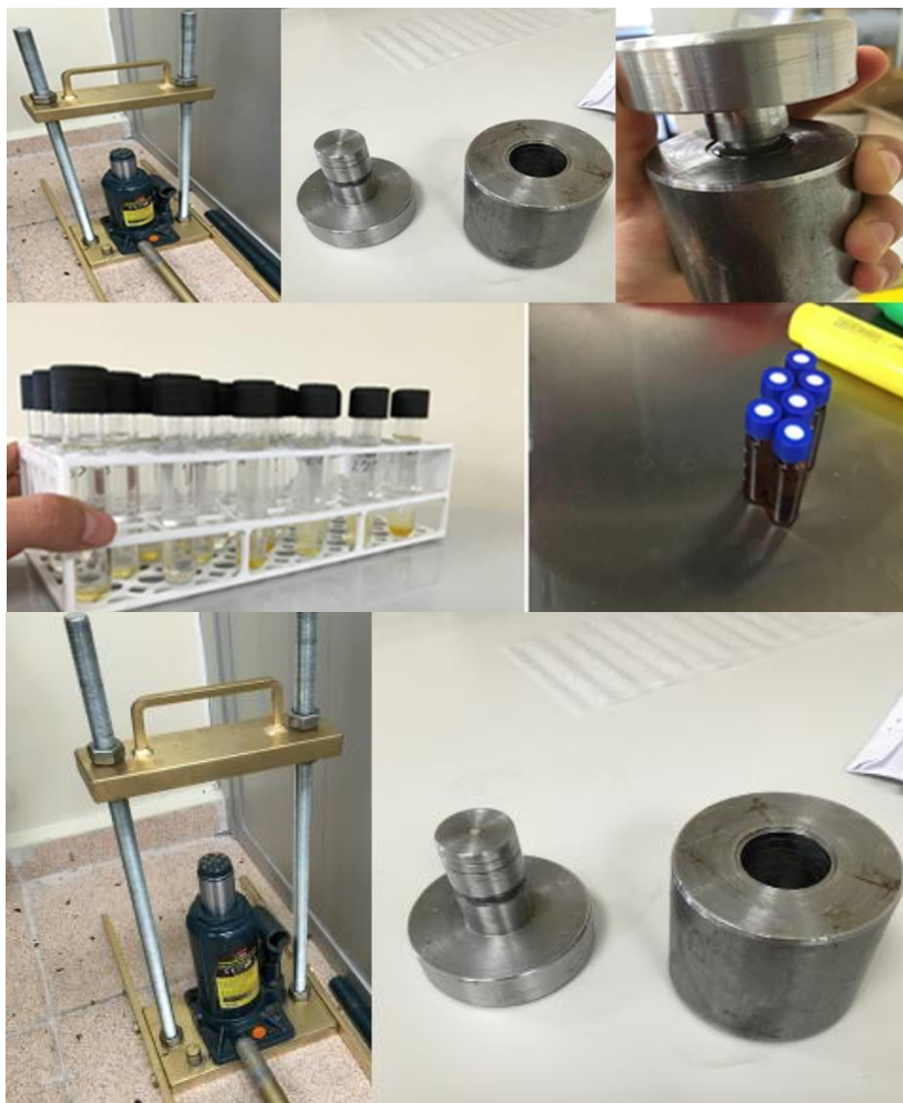
Figure 1. The cold press machine to get crude oil from sunflower seeds and obtaining samples for GC analysis
